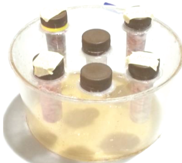
Plate 3.1: Locally Constructed phantom
